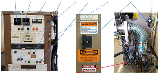
Fig 3 material research furnace shutdown procedure
